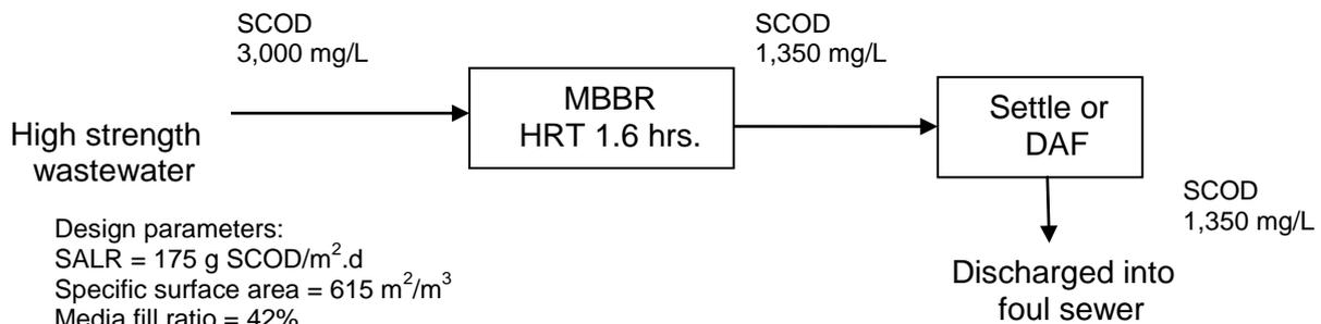
Figure 10: Treatment process using the new MBBR carrier
