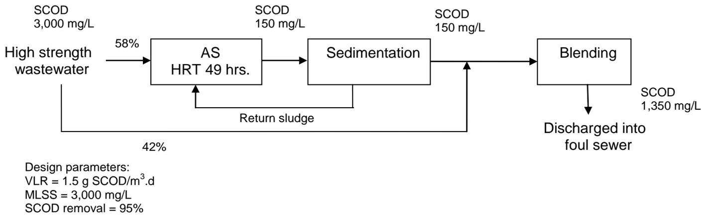
Figure 11: Treatment process based on activated sludge
