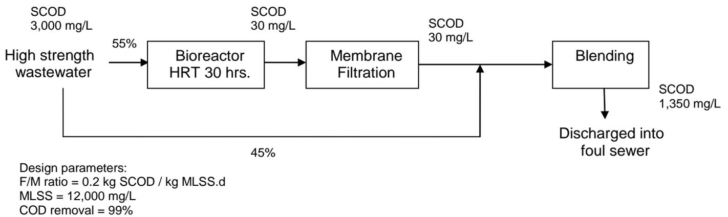
Figure 12: Treatment process based on MBR technology
